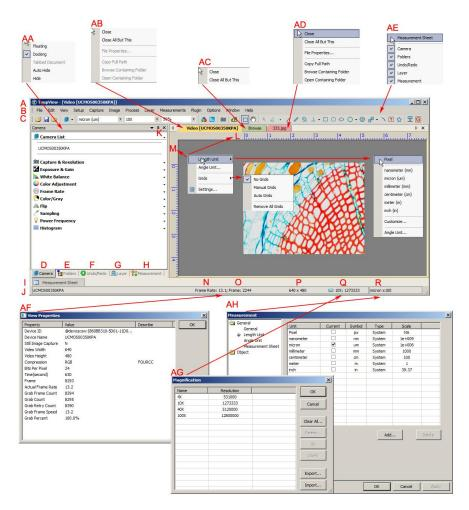
A:ToupView; B: Menu; C:ToupView toolbar D:Camera Sidebar ; E: Folders Sidebar ; F: Undo/Redo Sidebar ; G: Layer Sidebar ; H: Measurement Sidebar ; I: Measurement Sheet; J:Statusbar; K: Auto Hide button L: Horizontal ruler; M:Vertical ruler N:Frame Rate O:Frames captured P:Current Video sizes
