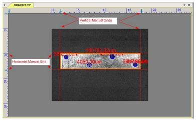
Choose the Grids>No Grid command to remove the Manual Grids overlaid on the video/image window. The menu will be checked.
