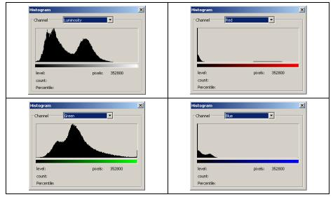
If the image is RGB true color, choose R, G and B to display a composite Histogram of the individual color channels in color.
