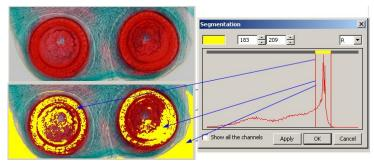
Choose the Segmentation command on a True Color image, select either Red(R), Green(G), or Blue(B) channel to do the operation.
