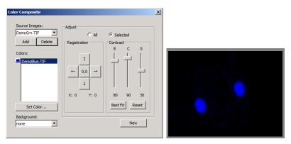
You can combine gray-scale images into a color composite. Any group of gray-scale images that are of the same size can be mixed in a color composite. Images of 8-, 12-, 16-bit integer or floating point format are combined into a 24-bit color composite. Each input channel will have individual LUT adjustments, as well as a registration offset to line it up with the rest of the images.
