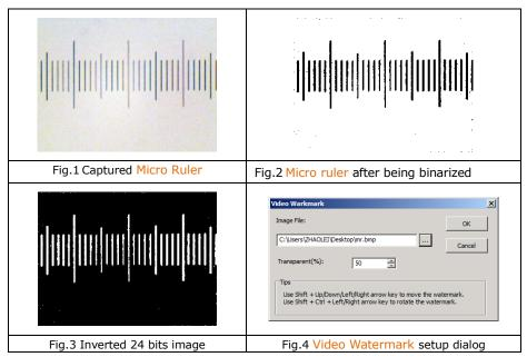
4. Choosing the Setup>Video Watermark••• command and a dialog called Video Watermark is brought up as shown in Fig.4. Click the 🔜 button to locate the image saved in step 3. Use the defaults Transparent (%)(50). If everything is ok, click OK button. The final Video Watermark is overlaid on the video window as shown in Fig.5.
