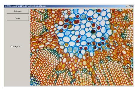
In this dialog, video Resolution can be selected (Combobox if it has). The Video Source Property can be set by clicking the Setting••• button. Click the Snap button to capture an image. This will create a new window and its title bar will be assigned a digital as the image window name;
