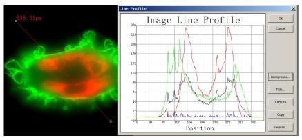
Line Profile: In a Line Profile, the X-axis represents the spatial scale, and the Y-axis represents the intensity values which range from 0 to 255. If the image is a gray scale image, the gray value will be profiled. If the image is a RGB color image, the R,G and B values will be profiled separately with the corresponding R, G and B colors
