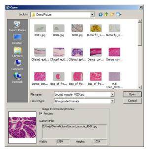
More than one image can be opened within ToupView simultaneously by a) with Ctrl + left mouse button method and b) Shift + left mouse button method to highlight the files to be opened;
