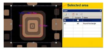
Note: Only when a ROI is selected and the Current item is checked on the Background in the Layer Sidebar, the Edit>Copy command can copy the selected image ROI to the clipboard.
