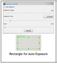
1. When the Exposure & Gain group is expanded, a green rectangle marked with "Exposure" will be overlaid on the video This marked region is a reference region for judging if the image brightness reach to the Exposure Target value. Drag or resize the Exposure ROI to the dark area will increase the video brightness and drag it to the brighter area will decrease the video brightness;
