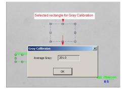
2. Choose the Edit>Image Select command or click the Image Select button and the toolbar to select a reference region, and choose the Setup>Gray Calibration... command. A dialog called Gray Calibration will be brought up to display the current ROI Average Gray. Now the brightness of the microscope can be adjusted until the Average Gray reaches to the desired value. Click "OK" to finish the calibration and return to the application area. The desired value here is around is 200.
