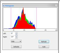
1. A Histogram illustrates how pixels in an image are distributed by graphing the number of pixels at each color intensity level. The Histogram shows detail in the shadows (shown in the left part of the histogram), midtones (shown in the middle), and highlights (shown in the right part). A Histogram can help you determine whether an image has enough detail to make a good correction;
