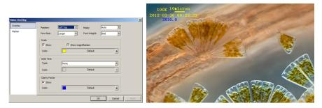
This command will invoke Overlay page as above. The Position, Font Size, Font Weight of the Scale, Magnification and Date, and Clarity Factor can be defined
