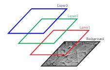
You use layers to perform tasks such as perform the measurement on the image without polluting the image and save it for the future adjustment for the further analysis, adding text to an image, or adding vector graphic shapes.
