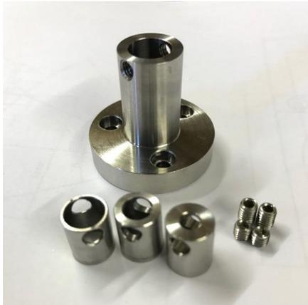
Slip the spacer Inlay over the worm and align the holes with the threads in the coupler, so the screws are able to contact the worm directly. Using the proper length hex screws (2 pcs, 180° positions) fix the coupler to the worm, but at first not tightly. Move the focuser worm manually to let the coupler align with the worm, when done only then fix the coupler to the worm tightly, and the motor to the worm housing.
